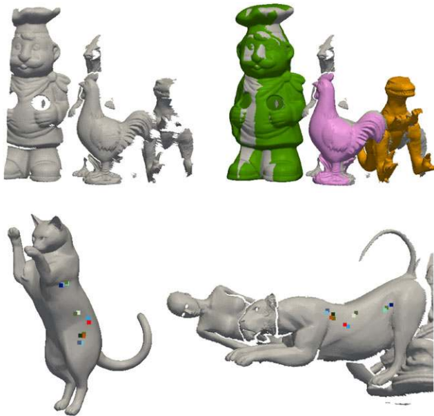
Fig. 9 Two examples of mismatches generated by our method; in the first case the dinosaur in the back was not detected and matches were not generated at all, the occlusion and clutter being respectively 91.4 % and 91.9 %. In the final example the cat model has been erroneously matched (false positive), due to very similar descriptors being present in the scene (Color figure online)
