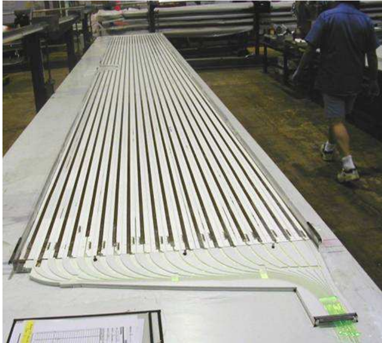
Figure 3.5: A diagram of a MINOS scintillator module
