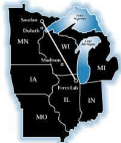
Figure 3.1: A geographical picture of the MINOS experiment. Neutrinos are produced at Fermilab and go through the Near detector, measuring the unoscillated energy spectrum, then the neutrinos travel 735 km to Soudan mine to be detected, in their oscillated form, at the Far detector.
