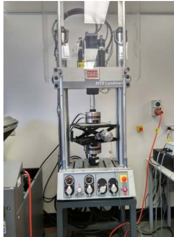
Fig.3. Test system for seat suspension
