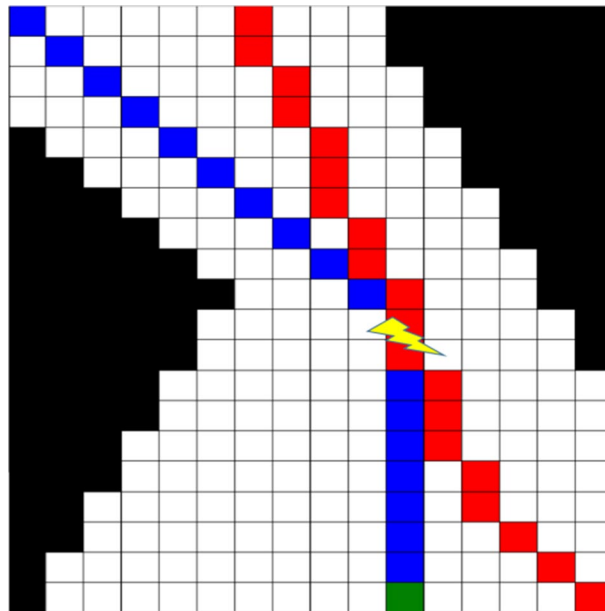
Fig. 15 Path planning results of traditional A* algorithm. The experimental results of the traditional A* algorithm are shown in this figure. We can observe that the traditional A* algorithm can avoid all static obstacles well, and the path length is optimal. However, it is difficult for traditional A* algorithm to effectively avoid the straight ships whose position changes dynamically in each round, resulting in the collision between the give-way ship and the direct-sailing ship at the yellow sign
