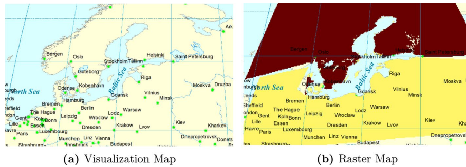
Fig. 3 Visualization map and raster map of the Baltic Sea geographic information. The rasterization method can represent geographic entities more effectively than the vector data method
