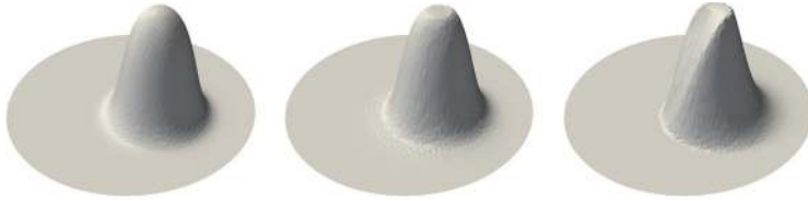
FIG. 1. Rotation of smooth data, unstructured mesh, 6773 \mathbb{P}_1 nodes, t = 4 . Exact solution (left), limiter solution with lumped mass matrix correction (center), and limiter solution with lumped mass matrix (right).
