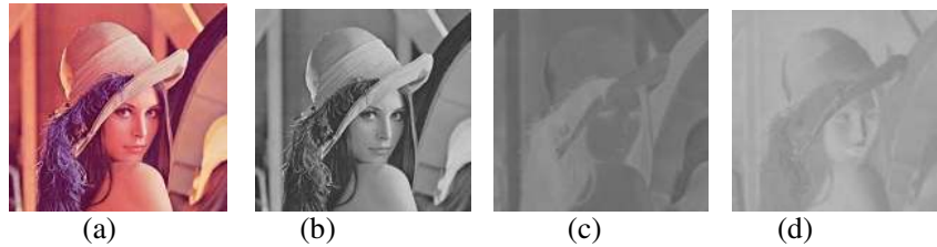
Figure. 2 (a) Lena, (b) luminance component Y of (a), (c) chrominance component Cb of (a), (d) chrominance component Cr of (a)
