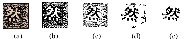
Figure 6: Processing style 2 images. (a) Original; (b) Binarized image; (c) Complement form; (d) After noise removal; (e) After cropping and rescaling
