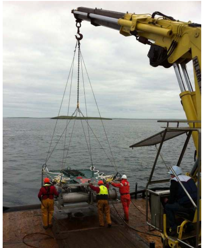
Fig. 5. Deploying the FLOWBEC frame. A complex arrangement of bridles is used to lower the frame to the seabed, before a surface-actuated hydraulic release leaves the frame on the seabed in 20 min with no trailing lines—essential for surveys in tidal sites.
