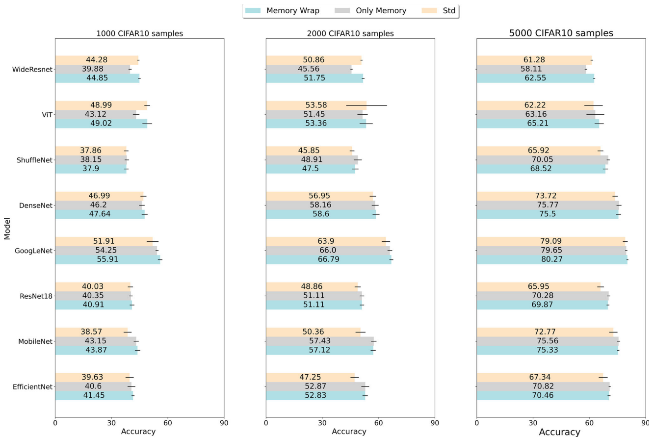
Fig. 7 Avg. accuracy and standard deviation over 15 runs of the standard model and two variants of Memory Wrap, when the training dataset is a subset of CIFAR10. For each configuration, we highlight in bold the best result and results that are within its margin
