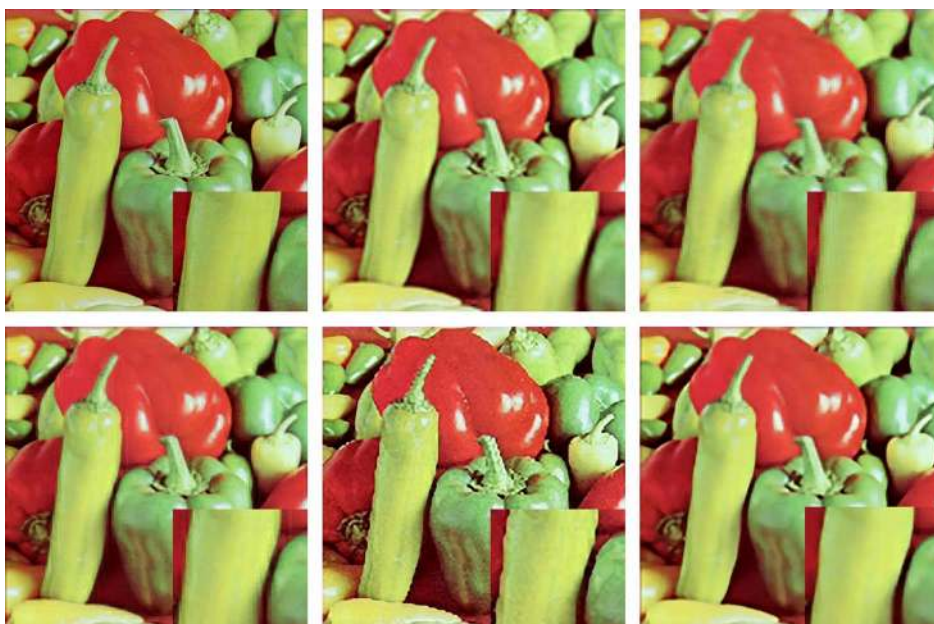
Fig. 8. Example SR results (with a magnification factor 4) and their PSNR values. Top row: ground truth HR image, bicubic interpolation (PSNR: 28.19), LLE [15] (PSNR: 26.85). Bottom row: Yang et al. [21] (PSNR: 26.12), Glasner et al. [2] (PSNR: 24.87), and ours (PSNR: 28.66). Note that nearest neighbor interpolation is applied to degrade the image resolution in this example.
