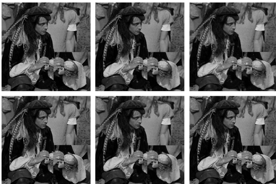
Fig. 9. Example SR results applying Gaussian blur kernels for degrading the image resolution. Top row: Ground truth image, bicubic interpolation (PSNR: 27.45), LLE [15] (PSNR: 24.05). Bottom row: Yang et al. [21] (PSNR: 27.83), Glasner et al. [2] (PSNR: 27.92) and ours (PSNR: 28.32).
