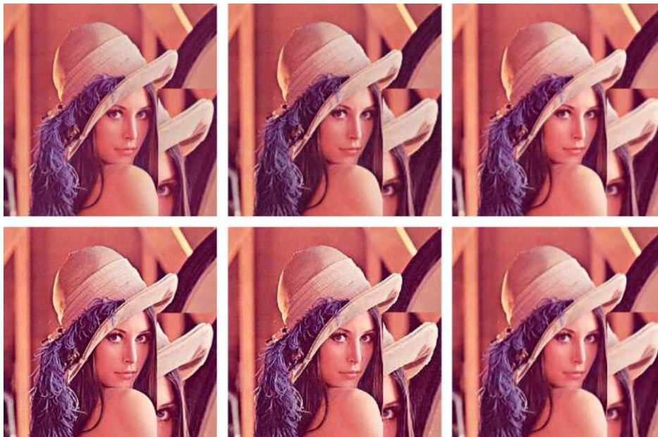
Fig. 7. Example SR results (with a magnification factor 2) and their PSNR values. Top row: ground truth HR image, bicubic interpolation (PSNR: 29.70), LLE [15] (PSNR: 27.43). Bottom row: Yang et al. [21] (PSNR: 28.86), Glasner et al. [2] (PSNR: 28.81), and ours (PSNR: 32.63). Note that nearest neighbor interpolation is applied to degrade the image resolution in this example.
