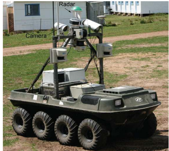
Figure 6. The CORD UGV used in this research along with its sensor suite.
