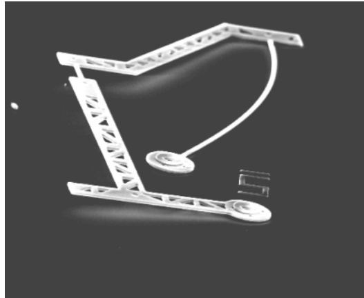
Figure 4-2 SEM of a Young mechanism experiencing the effects of pin joint clearances, as manifest by the out-of-plane deflection of the mechanism. The reaction force induced by the deflection of the slender beam (on the right) have resulted in the canting of the mechanism (see Fig. 4-1(f))
