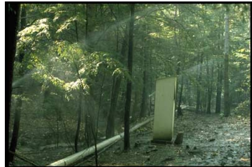
Figure 6. Spray irrigation devices are regulated to control the rate of irrigation under the tree canopy during the Shale Hills experiment.
