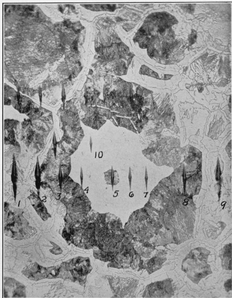
FIGURE 14.— Indentations in a quenched, high-purity iron—1.14-percent-carbon alloy (magnification, \times 250 ).
