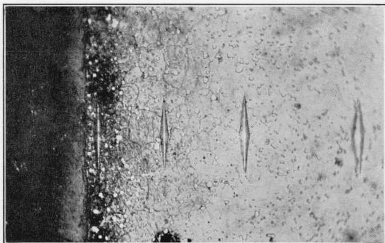
FIGURE 16.— Indentations in a specimen of nitrided hardened molybdenum-tungsten high-speed steel cut perpendicular to the nitrided surface (magnification, \times 500 ).
