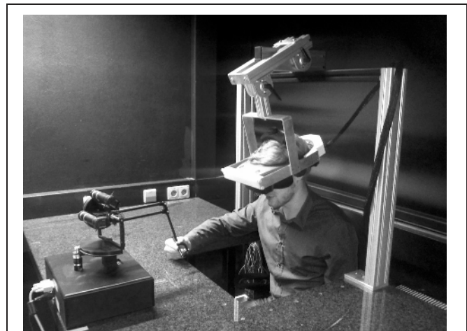
FIGURE 15 | Photograph of the experimental apparatus. The subject operates a Sensable® Phantom® Premium 1.5 High Force manipulandum and receives stereoscopic 3D visual feedback through an NVIS® nVisor ST50 head-mounted display.
