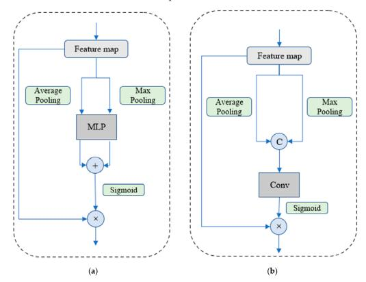
**Figure 2.** Network architecture of channel attention block (**a**) and spatial attention block (**b**). The channel attention block learns which channels of feature maps are important; the spatial attention block finds out "where" feature maps are vital. Together, *MAB* can aggregate more effective information regarding categories.
