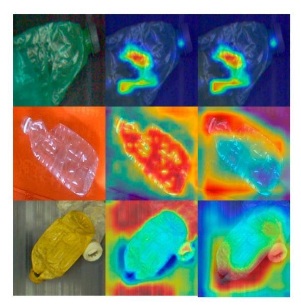
**Figure 4.** One bottle image (on the left) and its grad cam map of a waste bottle with the damaged classification on the last layer of RB (in the middle) and on the last layer of *MAB* (on the right). Our model can precisely locate the "damaged area" and the *MAB* makes it more focused (we mark relatively unimportant pixels for classification in blue and relatively important ones in red).
