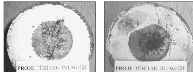
Figure 7—A harzburgite (left) and a high-grade chromite (right) sample after indentation testing
