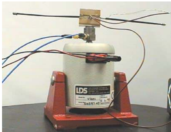
Figure 31 The SMA test rig: the SMA TVA is attached to the shaker through the impedance head
