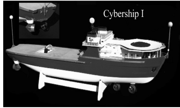
Fig. 4. Cybership I [11], supply vessel scale 1:70.
