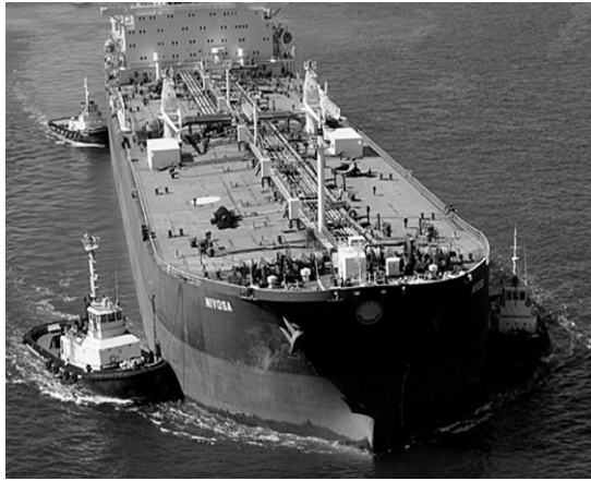
Fig. 1. Ship berthing with assistance of tugboats.
