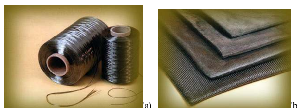
Figure 4. (a) Basalt fiber (b) Preforms for composite
