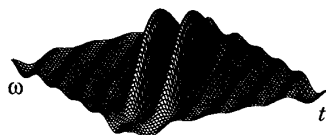
Fig. 11. OK TFD of the chirp signal of Fig. 1(b) computed using the untapered optimal kernel. Compare to Fig. 8(c), and note the substantial ringing that occurs without tapering.
