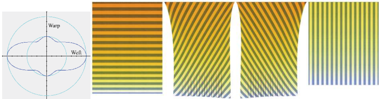
Figure 4: A large square piece of cloth cut along various fiber directions, hanging attached at one edge. The material is linear anisotropic (3), with 2 E_{uu,uu} = 1 E_{vv,vv} = 8 E_{uv,uv} (radial elongation stiffness diagram far left). This represents typical anisotropy of cloth materials, which usually have a much lower shear/elongation stiffness ratio than isotropic materials. Strips show weft fiber direction. Colorscale shows average tensile strain.
