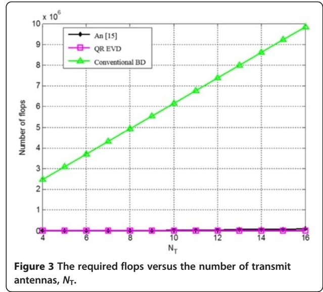
Figure 3 The required flops versus the number of transmit antennas,  $N_T$ .
