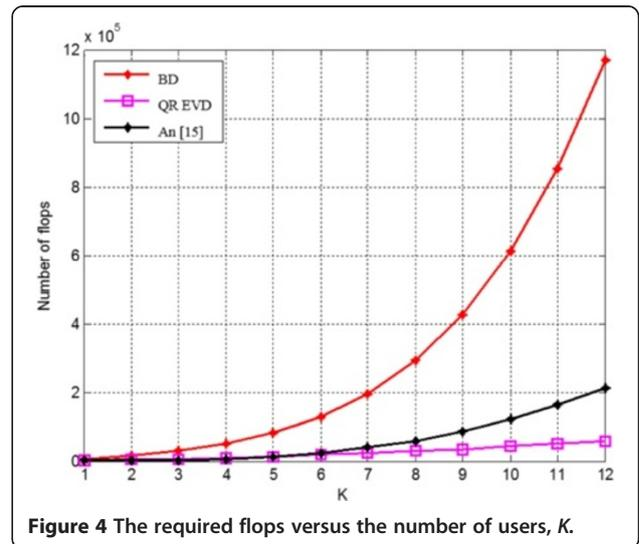
Figure 4 The required flops versus the number of users,  $K$ .
