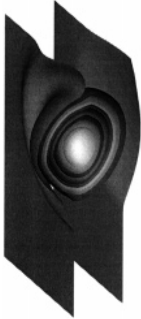
FIG. 10. Contours of the density at the beginning of penetration of the copper sphere into water.
