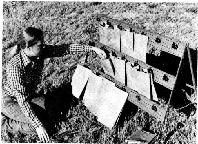
Fig. 1. Sack-holding frame, made with angle iron and pegboard, holds and organizes sacks.
