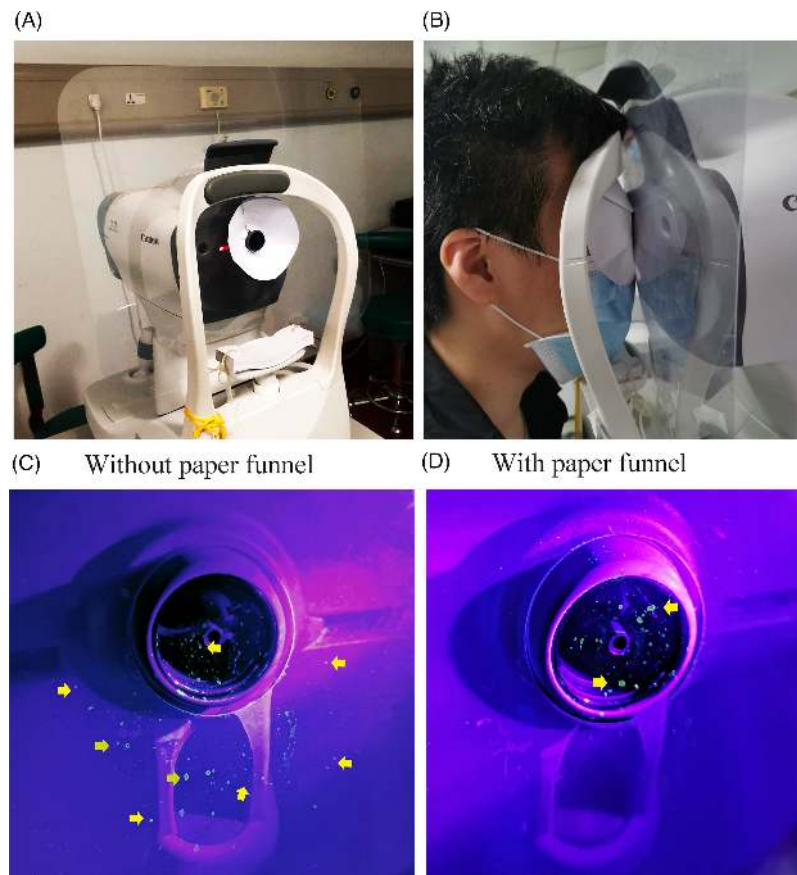
Fig. 1. The screening of the scattered droplets with fluorescent dye on the NCT machine with the novel protective measure. (A) A transparent plastic shield (41 cm × 36 cm) and a homemade paper funnel were installed on the NCT machine. (B) The volunteer positioned his head in the chin and forehead rest, and his eye was covered by the funnel. (C) Scattered tear droplets on the shield and sensor with the plastic shield only (yellow arrow). (D) Scattered tear droplets on the sensor with the plastic shield and the paper funnel (yellow arrow).
