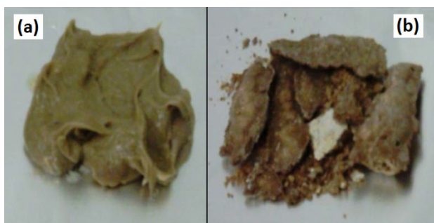
Figure 1. Raw material pretreatment: (a) crude rice bran oil soapstock (RBOS); (b) RBOS after saponification and drying steps
