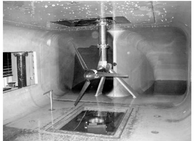
Fig. 13. Marine turbine tested in [39]. (Illustration reproduced with the kind permission of the authors.)
