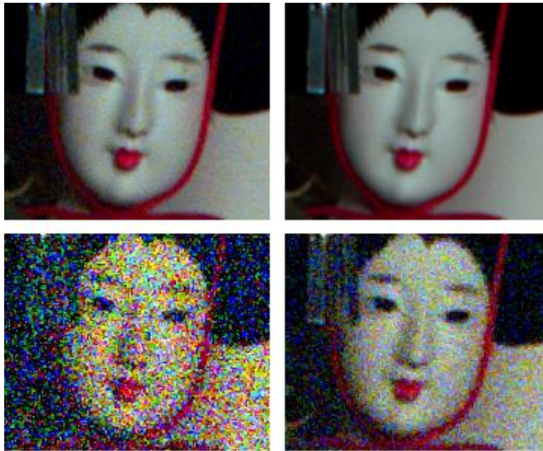
Figure 5. Simulations illustrating the benefits of correlated double sampling (CDS) at different levels of sensor irradiance (see text for details).
