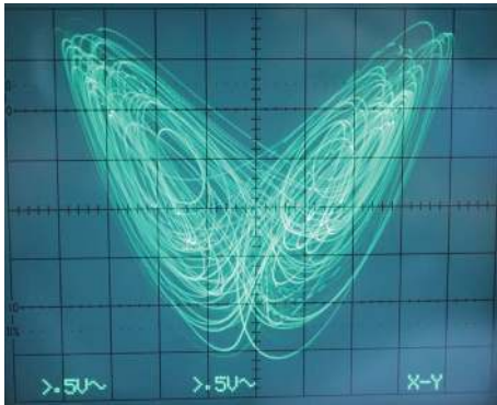
FIGURE 14: Circuit implementation result of two-wing hyperchaotic attractor.
