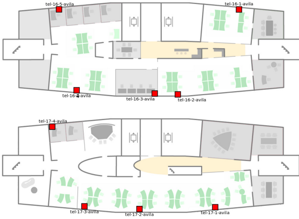
Figure 1: The BOWL indoor testbed spans two floors. There are five nodes on the 16th floor (top picture) and four nodes on the 17th floor (bottom picture). The host names are indicated with the convention: tel-floor-node.
