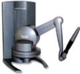
Figure 1: The Phantom Desktop provides one single point of contact to the user
