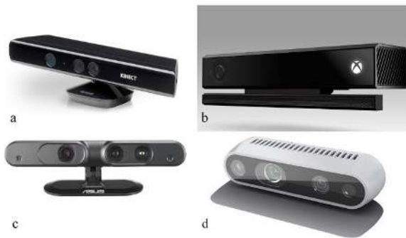
Figure 2. RGB-D cameras: (a) Microsoft Kinect v1, (b) Microsoft Kinect v2, (c) Asus Xtion PRO LIVE, (d) Intel RealSense D435
