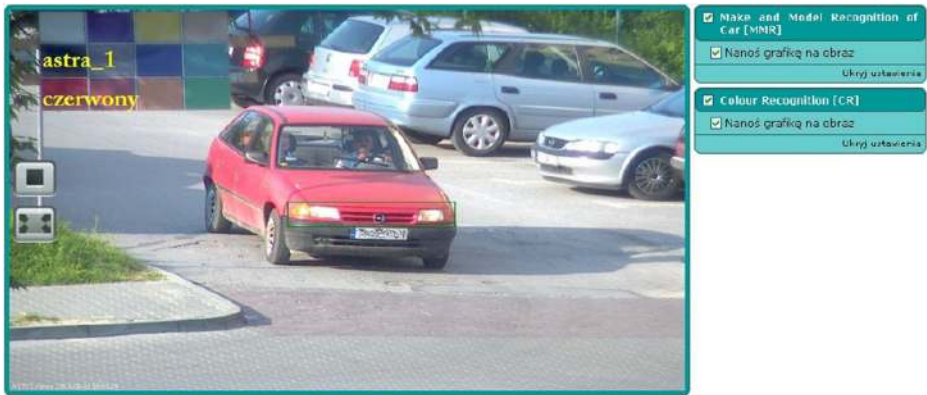
Fig. 4 Sample look of the iCamera User Interface (Captions “astra_1” and “czerwony”, displayed at the top left of the screen are the metadata returned by the MMR and CR modules, respectively. Because the LPR module is off at the moment – it has been deactivated using checkboxes situated at the top right of the screen, there is no information about registration numbers
