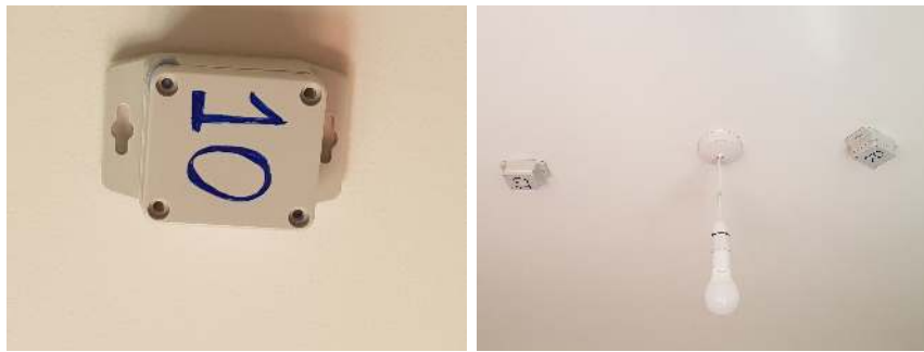
Figure 7. A BLE (left) and a set up in a room ceiling (right).
