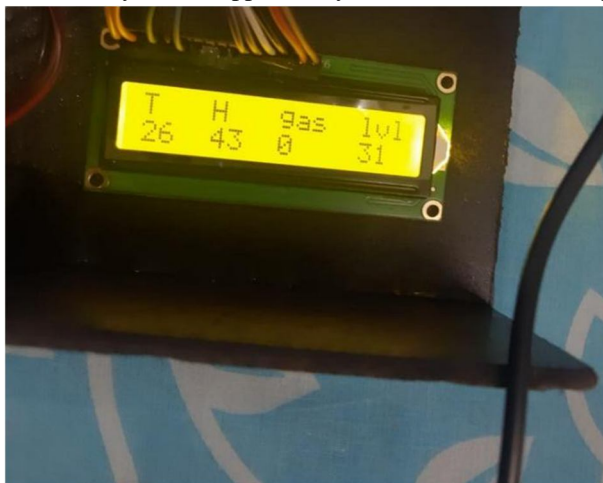
Fig. 6 LCD display showing various readings
