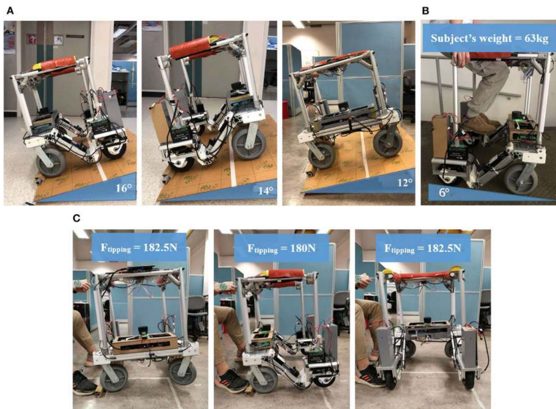
FIGURE 6 | Stability tests; (A) Static stability test, from left to right: forward, backward, sideways; (B) Dynamic stability; (C) Tipping resistance test.
