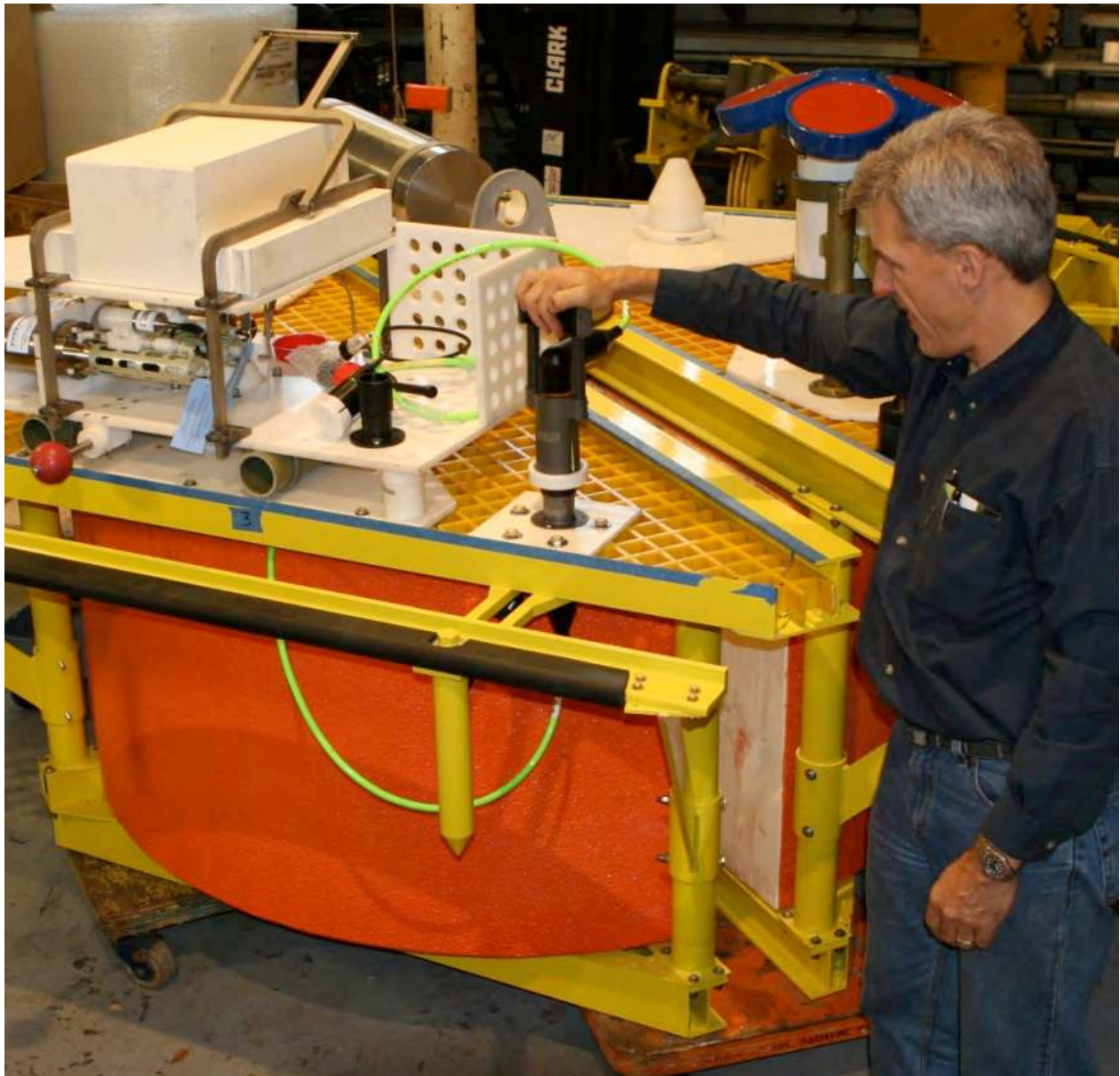
Fig. 9. The subsurface float. The instrument module with two CTDs is on the left; TM is plugging in the ROV mateable connector, connected to the secondary node in the left background. The ADCP is top right. A titanium post fits into the slot in the float.
