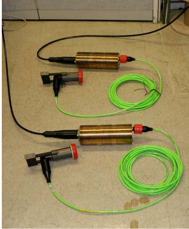
Fig. 3. ROV-mateable connectors and the electro-optical converters (in beryllium copper pressure cases) attached to each end of the (black) seafloor cable.
