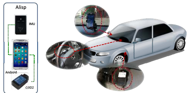
Figure 2. Overview of the Android-based in-vehicle sensing platform
