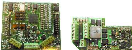
(a) Module controller board. (b) DC/DC board.
