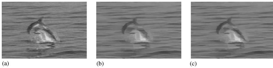
Fig. 2. Frame pre-smoothing with the proposed ASF: (a) original frame; (b) filtered frame with structure elements of 4 orientations; and (c) filtered frame with structure elements of 8 orientations.
