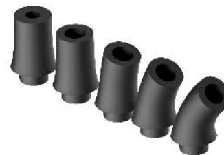
Fig. 3: Nozzles used to modify the propulsive characteristics of the baseline vehicle. Two left-most nozzles are straight and of varying internal diameter, the remaining ones are angled to deflect the direction of the jet and induce a turning moment.
