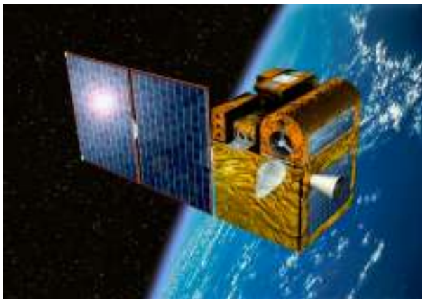
Fig. 1: Artist view of PICARD microsatellite, 60x60x80 cm 3 in size. Shown are the 3 instruments of the payload: SODISM, telescope and guiding, right, SOVAP, differential radiometer, center, and PREMOS (flux monitors) left, near the solar panels. In the back, one can see the electronics box supporting two S-band antennae and a solar pointer (acquisition maneuvers).
