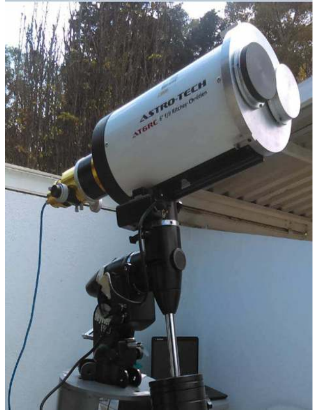
Fig. 1. The Solar Infrared Telescope with the housings for the germanium and Mylar filters at the aperture. The Mylar filter is used for visible light observations.
