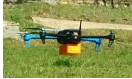
Figure 2. UAV and RFID reader
