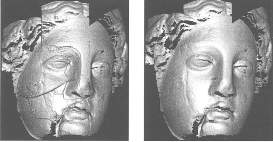
Fig. 2. The Greek bust after interactive (left) and global (right) registration of 12 scans.
