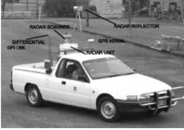
Fig. 2. The test vehicle, showing mounting of the MMWR and GPS systems.
