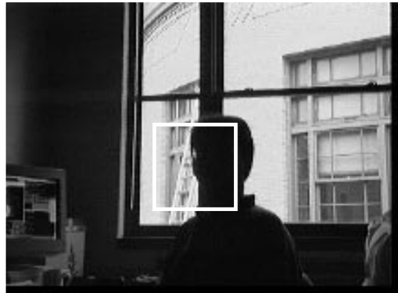
Figure 8: A scene with back lit objects as captured by a conventional CCD camera.
