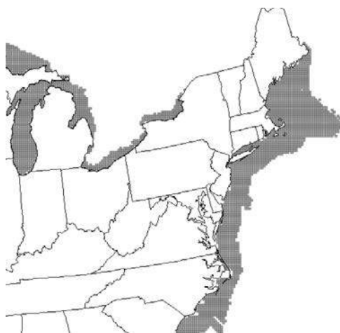
Figure 17. Wind project grid for the northeastern United States and Great Lakes regions (each region represents a potential offshore wind power project)
