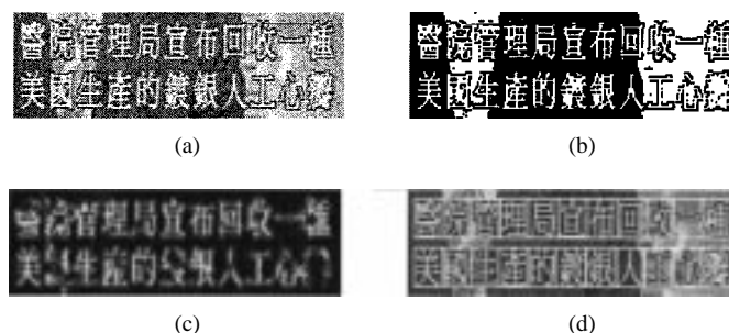
Fig. 8. Character segmentation examples. (a) Caption region. (b) Binary image. (c) Smoothed contour image. (d) Located individual characters.
